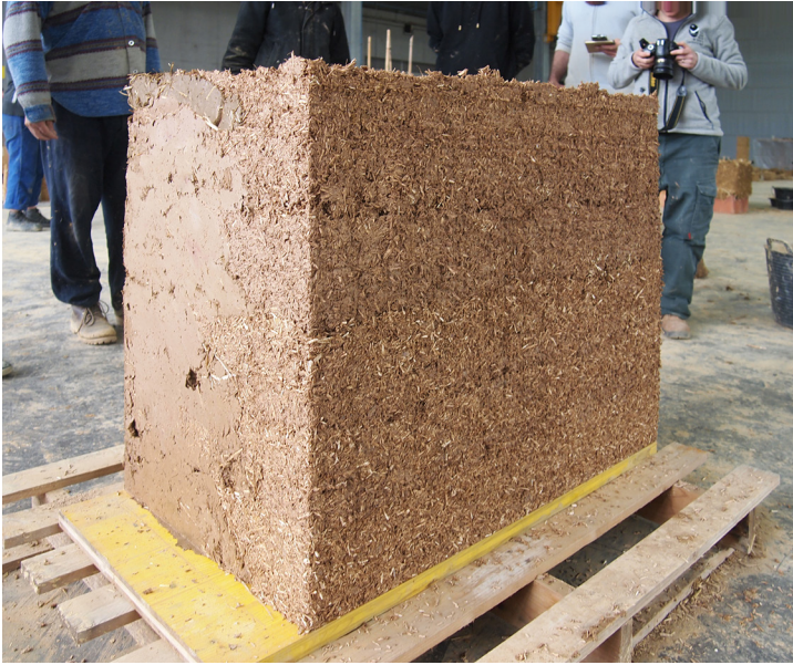
06 First test of the CobBauge construction process conducted in Les Grands Ateliers (Fr)
