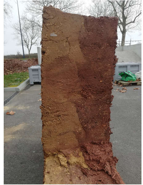
07 Test wall cut in ESITC, showing a strong bond between the cob and light earth
