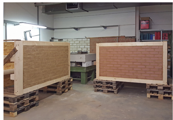
Earth block masonry test setup for tensile tests
