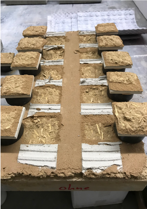
Testing tile bonding on an earth plaster substrate
