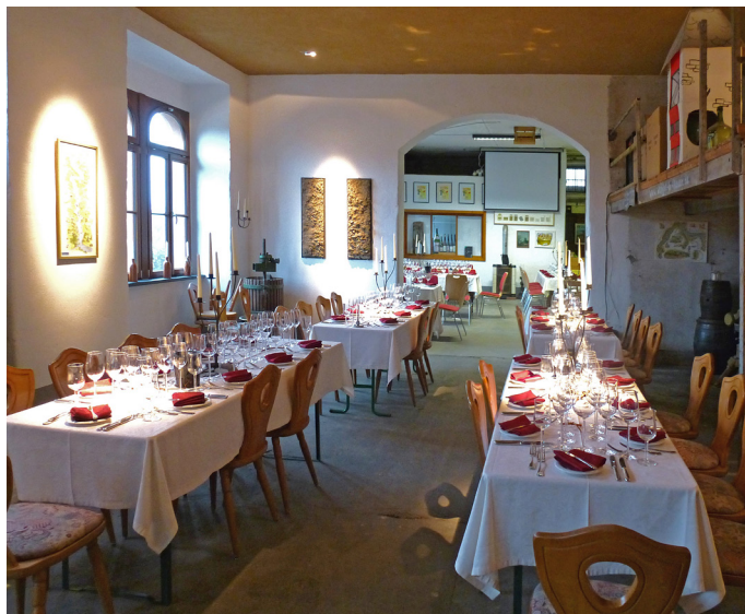
05 Interior of the wine tasting guestroom at Dr Kauer vineyard with the climate panel ceiling finished with earth plaster
