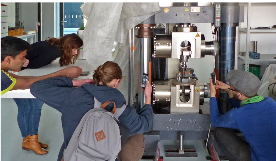
04 Self-produced adobe bricks on the test bench in the laboratory: Kompetenzzentrum Bau MV at Wismar University of Applied Sciences
